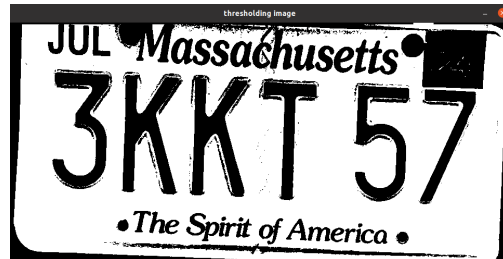
Fig. 20: OTSU Thresholding on Number Plate after Lumination Correction
